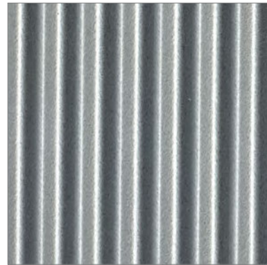
CORRUGATED GALVANISED ROOFING
