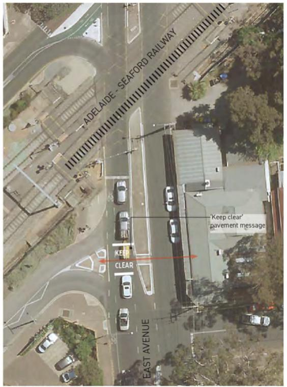
Figure 6.29 'Keep Clear' Pavement Message concept plan
