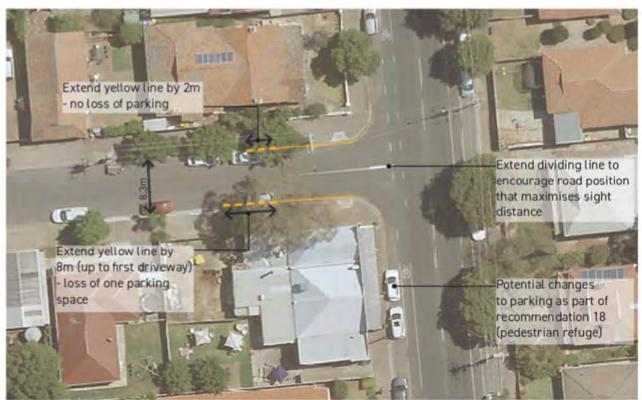
Figure 6.18 Recommendation No Stopping zone extension
